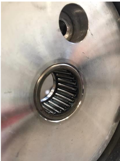
Needle bearing (Old situation)
