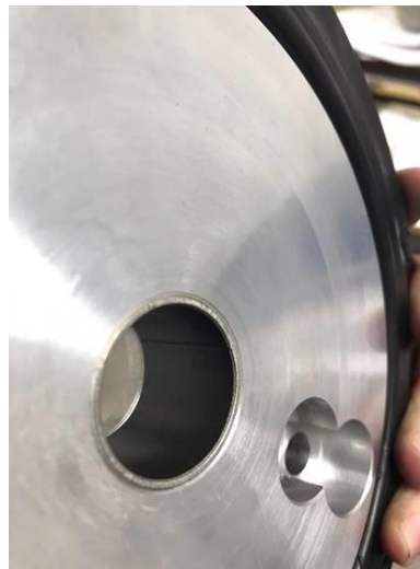
Slide bearing (New situation)
