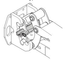
Connect the hydraulic hoses and any hoses for hammer lubrication (when fitting the hammer). Viewed from the rear, the tool's return hose must first be connected to the right side (A port) and then the delivery hose to the left side (B port).
