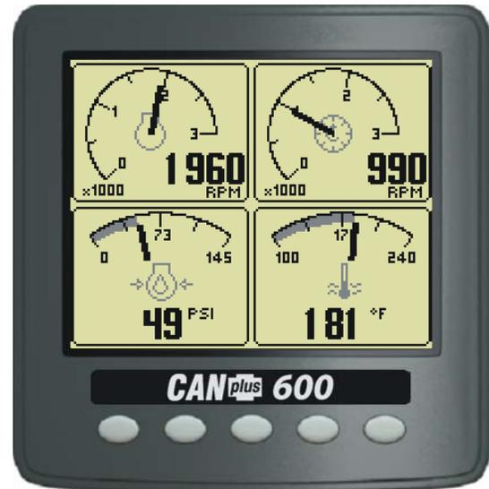
The other major design change is the Full Authority Electronic Engine Control. Engine performance is governed and monitored by an Electronic Control Unit (ECU). The diesel injector timing and duration is directly controlled electronically. The engine has no throttle cable or linkage. It has no mechanical governor. Electronic Engine data is collected and processed in the ECU and broadcast onto the Control Area Network Bus. (aka CANBus). The CANBus broadcast is to the SAE J1939 standard.
